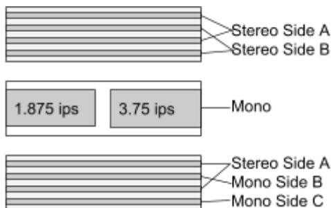
Three example layout of audio on an 1/4 inch tape.
