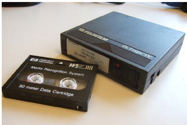
Figure 1: DDS-1 (left) and DLT-IV (right) tape
